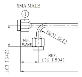
SMA Male to SMA Male cable assembly using ST085 Tight-Flex, Triple Shielded Coax, 6 inches long, Operating to 18 GHz.
